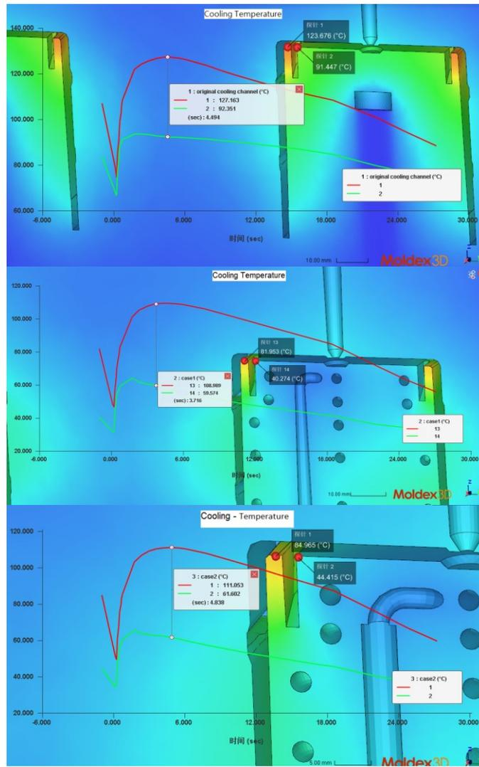
Fig. 10. Part surface temperature of conventional Cooling A1. The highest temperature is 127°C, the inner corner (Green line) highest temperature is 93.5°C. Part surface temperature of conformal cooling channel B1. The highest temperature is 102°C, the inner corner (Green line) highest temperature is 64°C. Part surface temperature of conformal cooling channel B1. The highest temperature is 111°C, the inner angle (Green line) highest temperature is 65.4°C.
