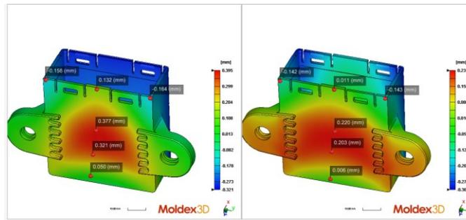
Fig. 12: Warpage analysis under A1 and B1 cooling channel simulation.
