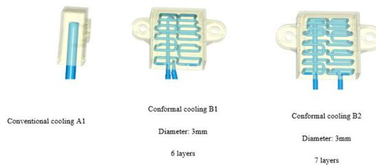
Fig. 7: Cross-section of conventional cooling channel (A1), TypeB1 and Type B2 conformal cooling channel.
