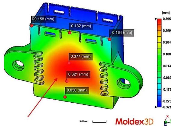
Fig. 3: Predicted location of deformation on car seat housing.
