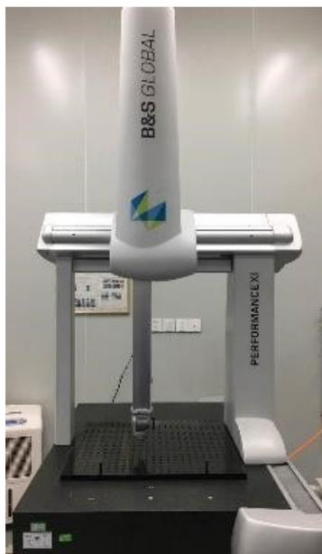
Fig. 2: Three-coordinate measuring machine.
